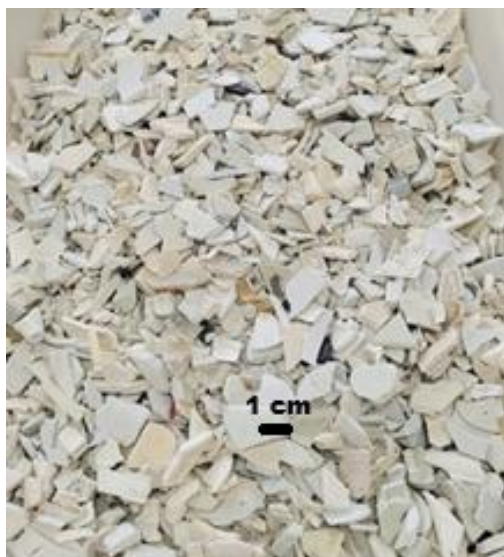
Figure 1. Polypropylene Plastic Waste Used in Research
